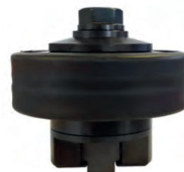
Test joint for IRTT-B
